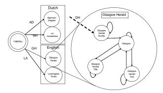
Figure 7: (Right) An example of part of the DFA CLEF2003. (Left) A close-up on the lexer for the Glasgow Herald Collection.
